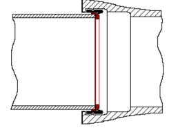
Push the spigot or "male" end of the pipe into the bell end, using minimal deflection and constant, steady forward pressure.
