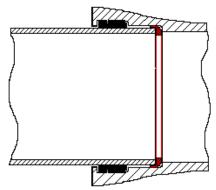
Press spigot or "male" end into bell end until the pipe is seated in its "home" position". Deflection may be used at this time, following pipe manufacturers' recommendations.
